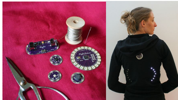
Figure 3. Components of the LilyPad Arduino (left) kit and a sample construction (right).
