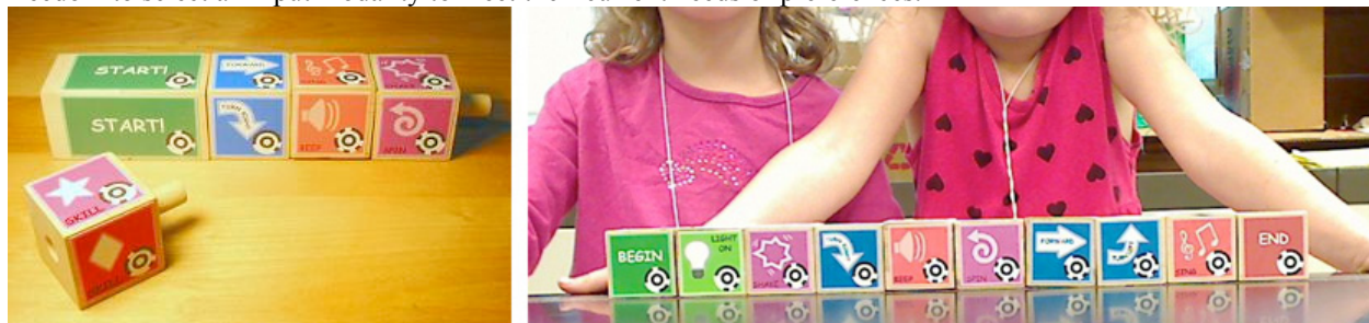
Figure 7. Tern allows children to program by connecting interlocking wooden blocks.
